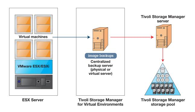
The Tivoli Storage Manager for Virtual Environments agent on a centralized vStorage backup server takes snapshots directly from the VMware server and transfers data to a server running Tivoli Storage Manager for placement and management in the storage pool.
