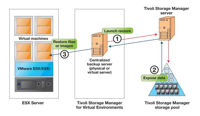
To restore files or volumes, the administrator launches a command on the vStorage backup server, exposes a snapshot that was saved in the storage pool, and maps the mounted data back to the virtual machine.
